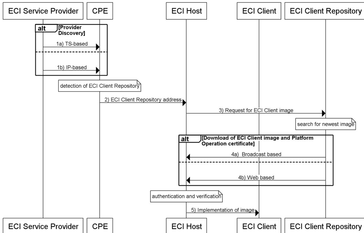
Figure 6-1: Flow diagram for the installation of an ECI Client
