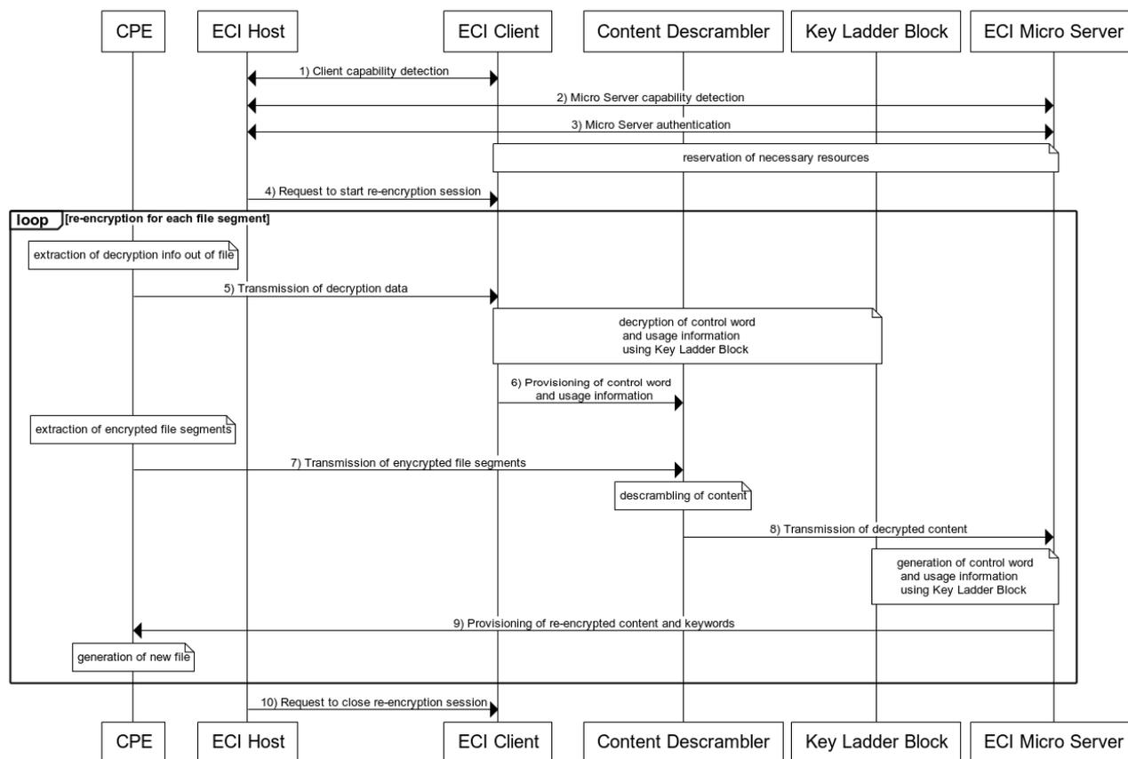
**Figure 9-1: Flow diagram for the re-encryption of content**
