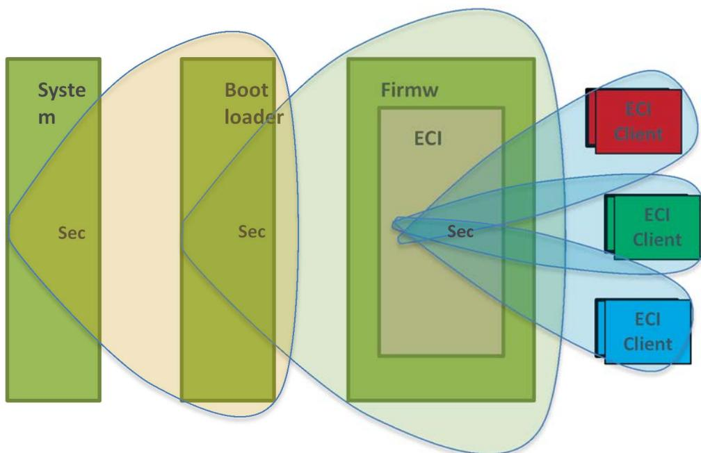
**Figure 11-1: Example for a chain of trust in an ECI environment**
