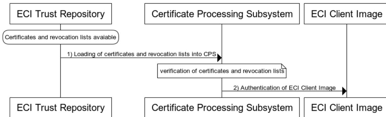
**Figure 11-8: Verification of certificates for the operation of an ECI Client**
