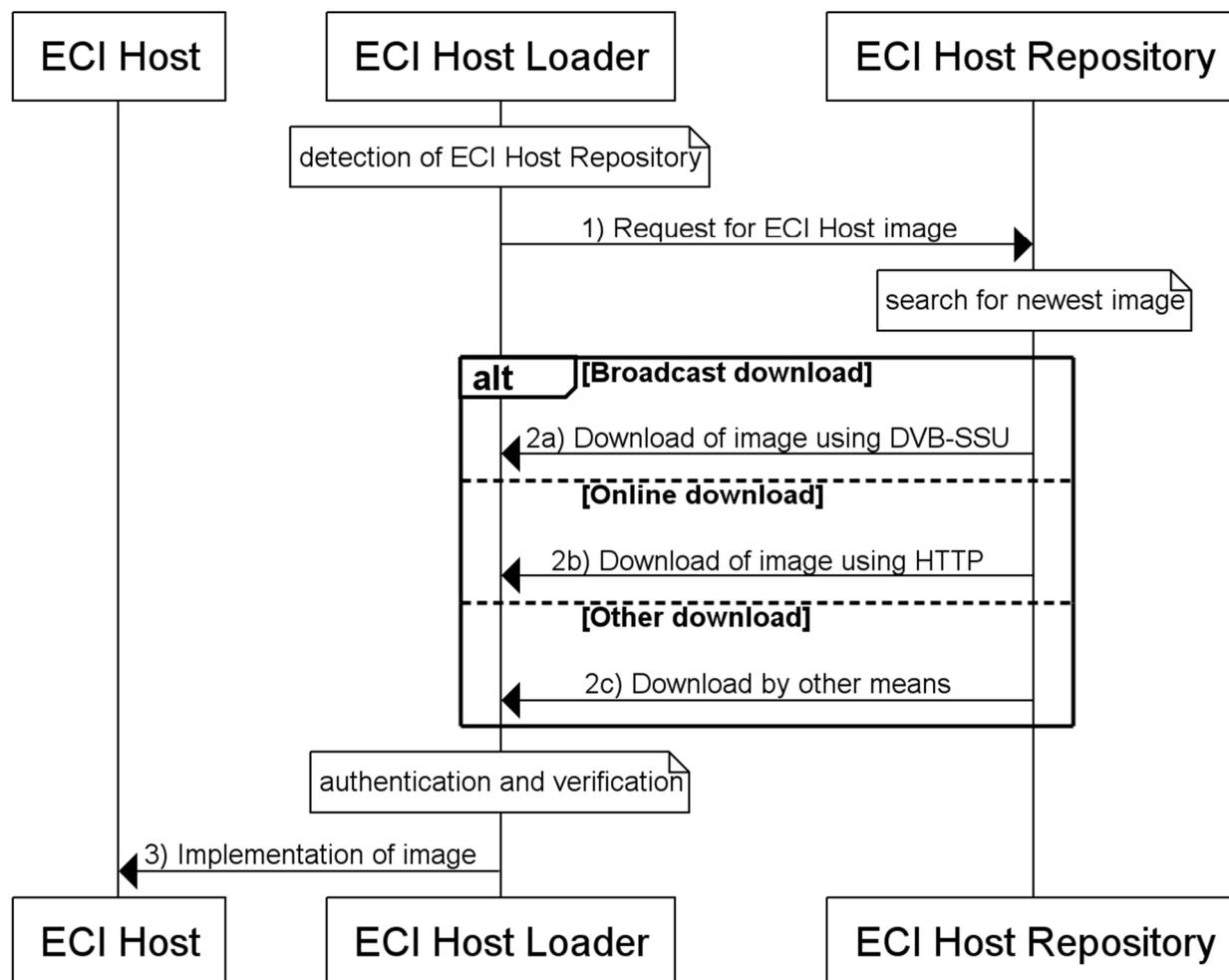
**Figure 5-1: Flow diagram for the installation of an ECI Host**
