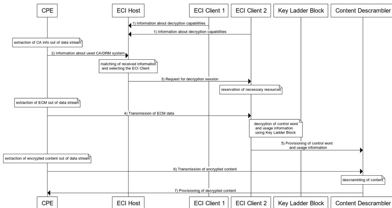
**Figure 8-1: Flow diagram for the decryption of content**
